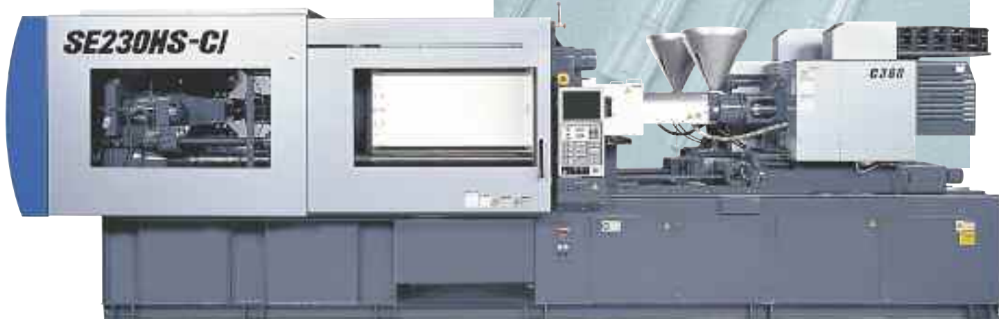
Sumitomo's new high speed double shot machine for packaging applications
